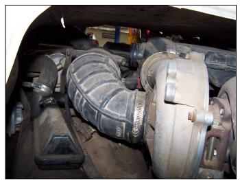
FIG 7: Turbocharger Inlet Hose and Crankcase Vent
