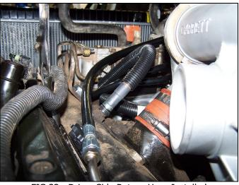
FIG 33: Driver Side Return Hose Installed
