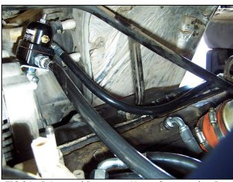
FIG 34: Driver and Passenger Hoses Connected to Reg
