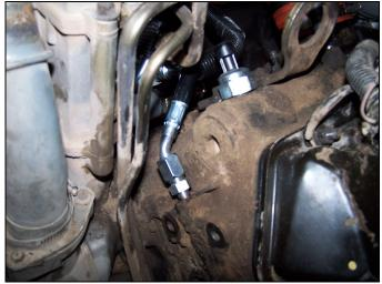
FIG 27: Drivers Front Feed Line Connected
