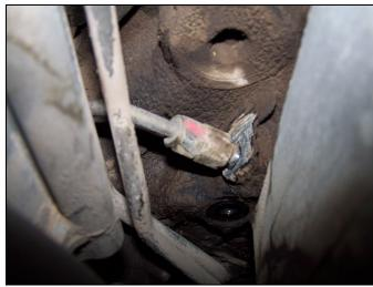
FIG 20 : Driver Front & Passenger Rear Fuel Line Example
