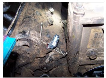
FIG 24: Passenger Side Front Fitting Installed
