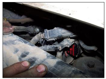
FIG 4 : Connectors Behind Cowl Wiring Harness
