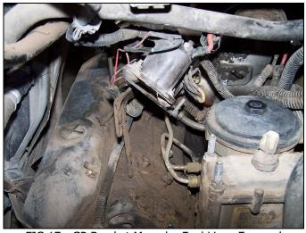
FIG 17: GP Bracket Moved – Fuel Lines Exposed
