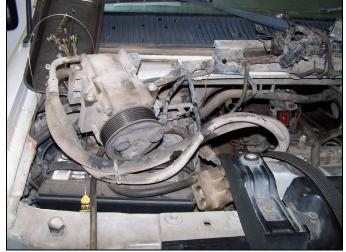
FIG 12: A/C Compressor Moved Off Engine
