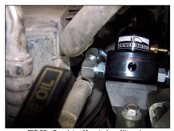
FIG 29: Regulator Mounted on Alternator
