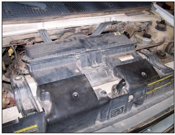
FIG 1: Airbox Lid and Lower Air Box
