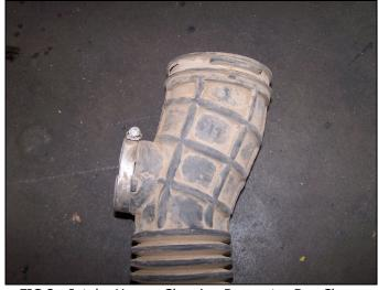
FIG 2 : Intake Hose – Showing Resonator Box Clamp
