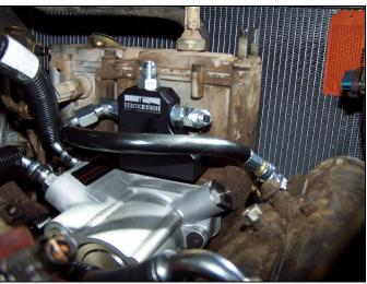
FIG 26: Fuel Bowl Delete Block Installed
