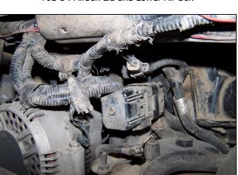
FIG 3: Main Engine Harness Connector
