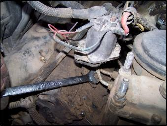
FIG 15: Wrench on Front GP Bracket Nut
