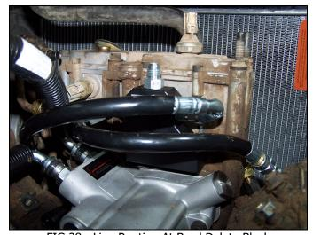
FIG 28: Line Routing At Bowl Delete Block
