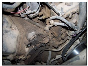
FIG 10: Alternator Bracket Removed
