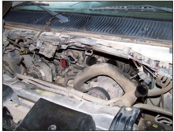
FIG 5 : Cowl Harness Pulled Up Out of Way
