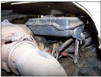
FIG 8 : Air Intake Resonator Box
