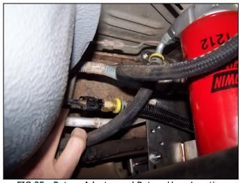
FIG 35: Return Adapter and Return Hose Location (NOTE: Current Configuration is a Black/Green Polymer Fitting with Directly Connected Hose)
