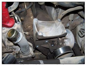
FIG 13: A/C Compressor Bracket
