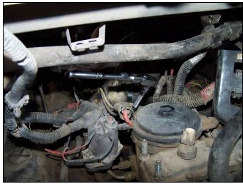
FIG 16: Ratchet on Rear GP Bracket Nut
