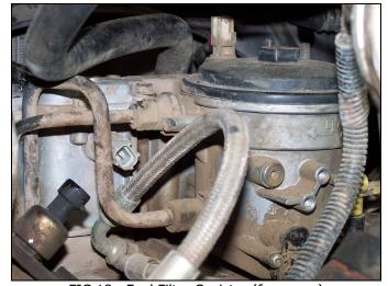
FIG 18: Fuel Filter Canister (from rear)
