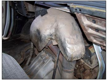
FIG 6 : Dog House Removed – Turbo Heat Shield Shown
