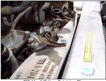
FIG 11: A/C Hose Retaining Clip
