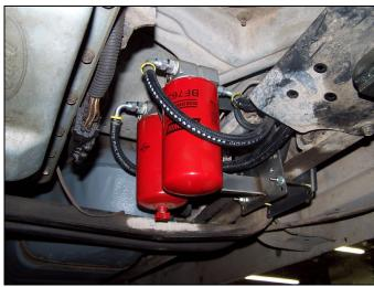
FIG 37: Driven Diesel Pre/Post Fuel Filter Kit
