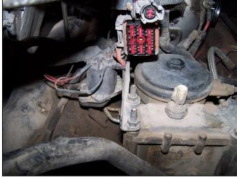
FIG 14: Wiring Harness Bracket on Reservoir
