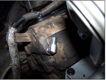
FIG 21: Driver Side Rear Fitting Installed
