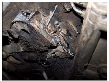
FIG 19: Passenger Front & Driver Rear Fuel Plug Example
